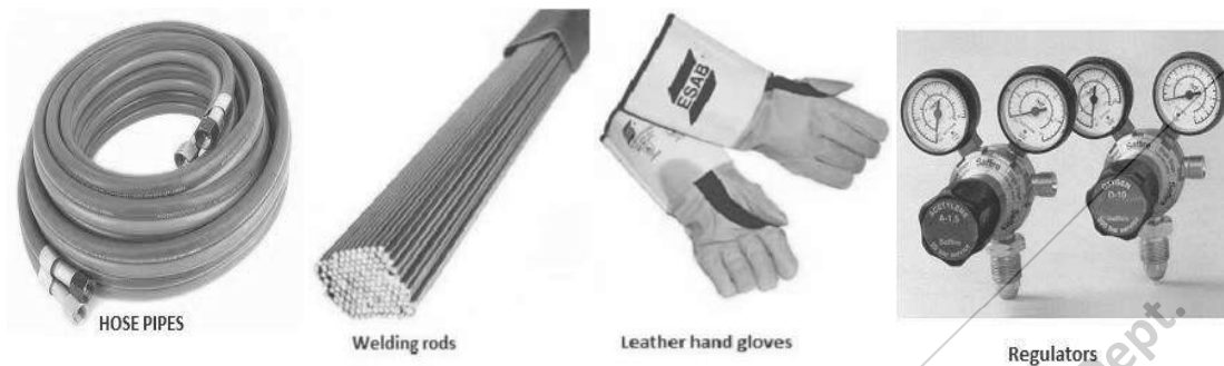
Fig. 3.6 Various Equipments of gas Welding
